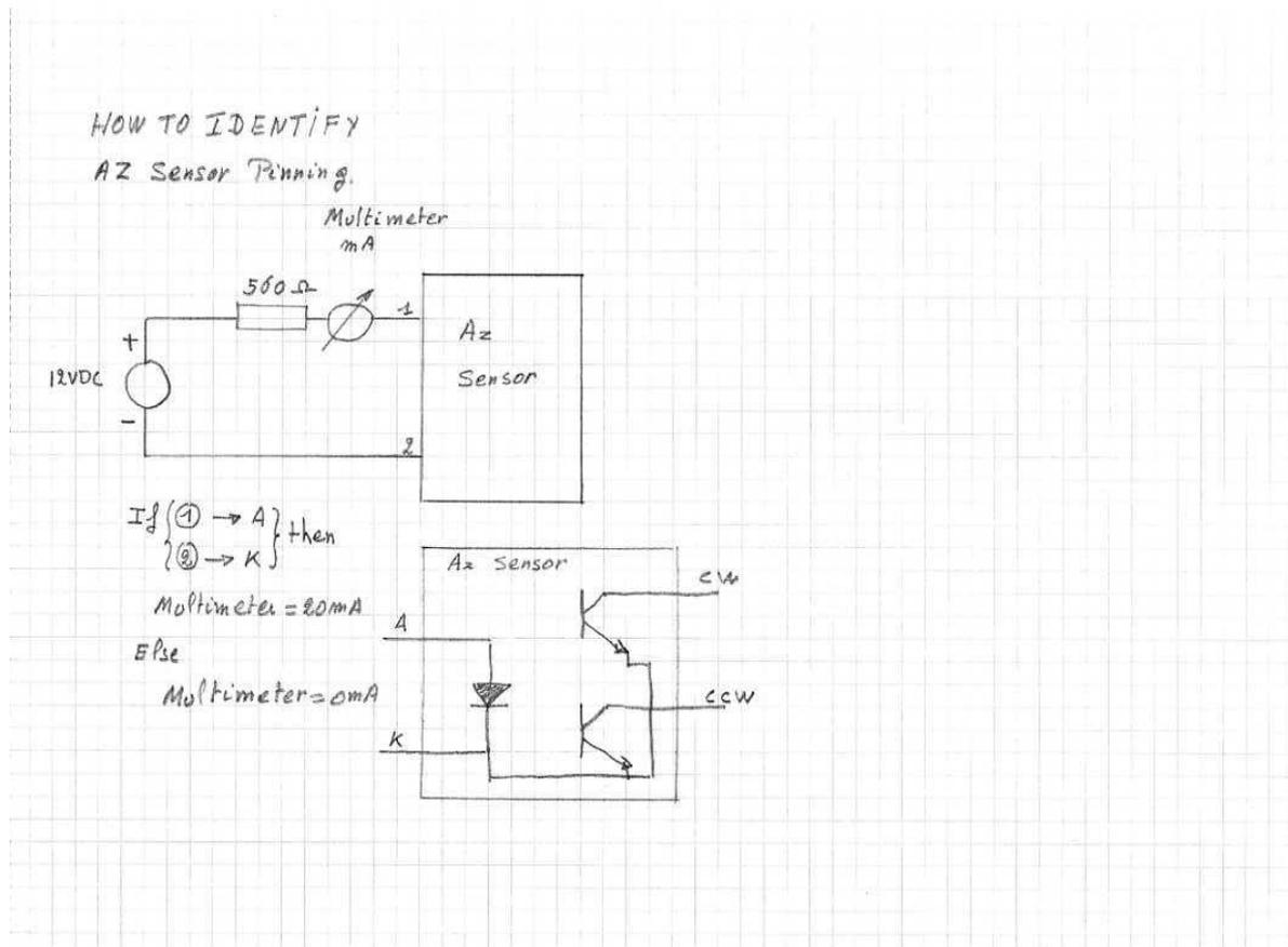
You need a Power supply of 12VDC, a 560 Ohm resistor (as usual to limit current in Azimuth sensor), a Multimeter to measure the current (available from RadioShark, an analog [\$10] or digital [\$30]).
