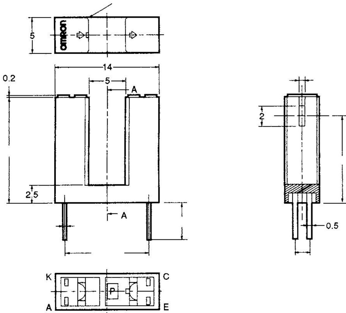
In one branch of the photo sensor a LED is generating light, which is detected by the photo sensor located in the other branch, provided there is no obstruction.
