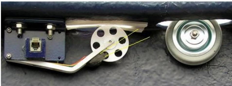
As the wheel is contact with the dome base, this wheel will rotate when the Dome is in move
