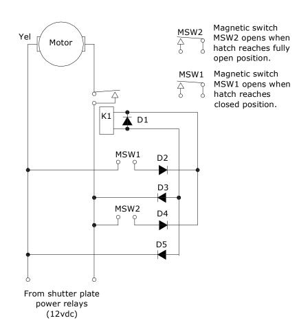
Note: When Yellow lead of shutter motor is positive, shutter moves to closed position.
