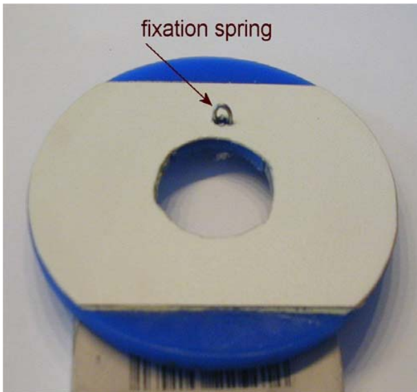
Figure 12, disk with magnets and fixation spring Covered with glued paper.
